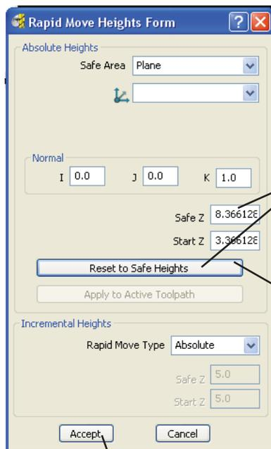
Click the Reset to Safe Heights, and the bit should move to the middle of the block and be above the block by the specified safe height.
