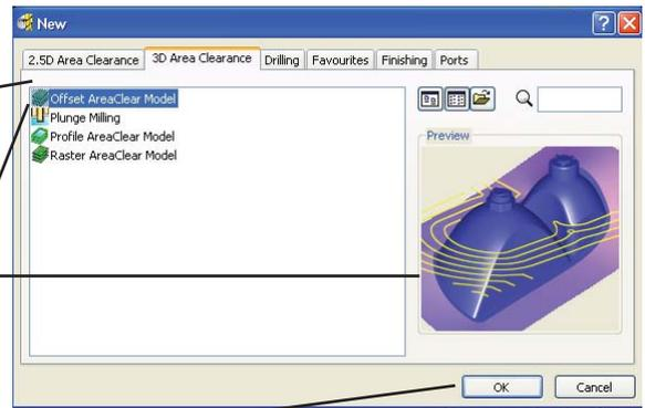
For Roughing a model, click the 3D Area clearance tab and then click on Offset Area Clear Model. A toolpath example will show up.
