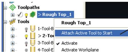
Right Click on the toolpath and choose Attach active tool to start. Your bit will jump to the starting point. If you click on the left or right arrows on your keyboard, the bit will follow the toolpath.
