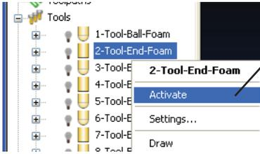
To make a tool active, right click on the tool you want to activate and select Activate. The tool will appear in the modeling window.
